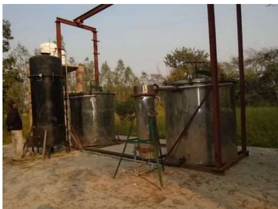
Figure 5: Mentha oil extracting unit (Steel Frame)
